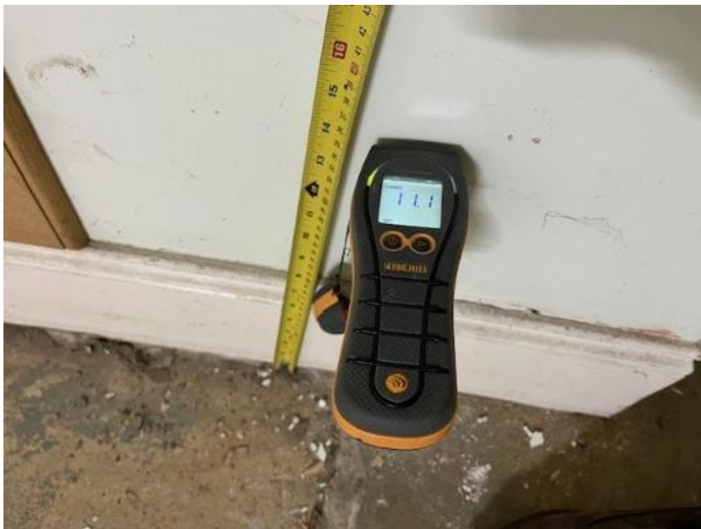
P73 – Moisture content reducing with height 11.9%
